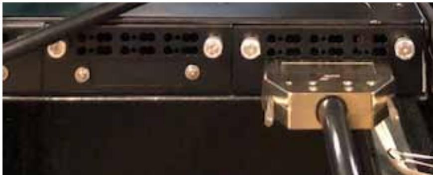
Backside of LCU with Signaling Y cable connected
